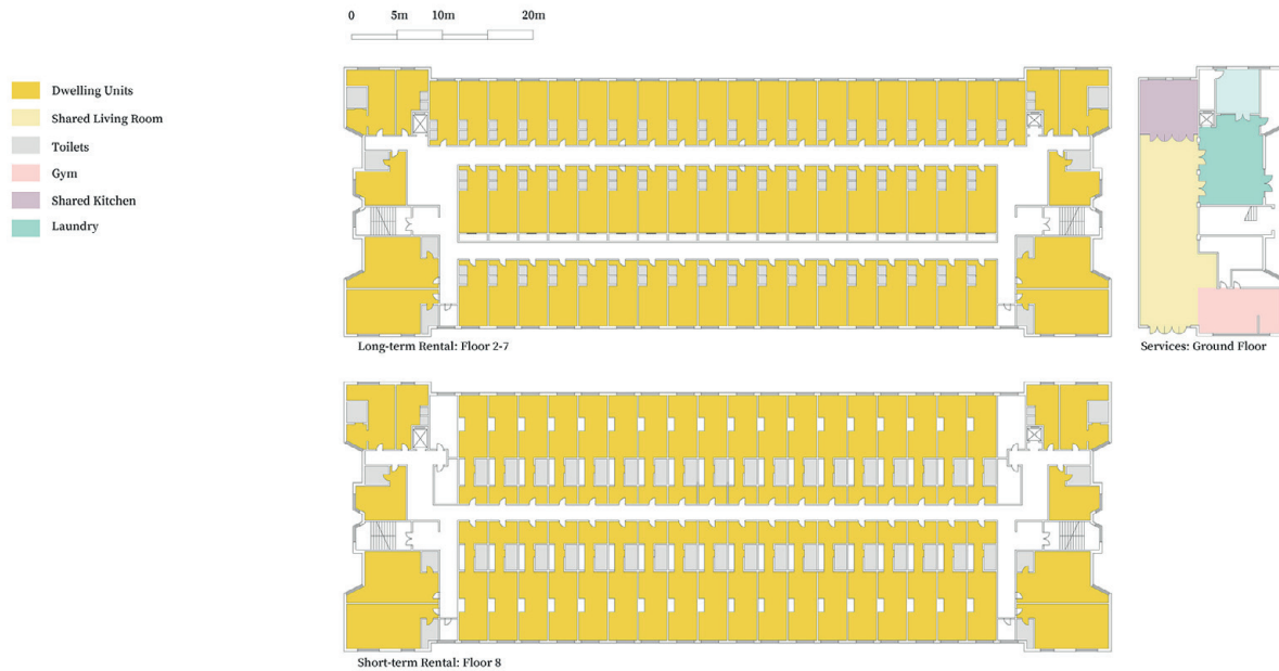
Figure 4. Apartment Layout of CJIA Apartment (Futian, Shenzhen), Drawn by the Author Based on the Baidu Satellite Map and Field Observations
